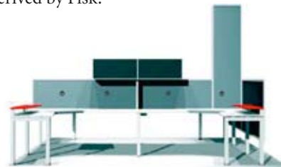
Figure 6 In this workstation, cooled fresh air is delivered via a vertical blade to a horizontal plenum, in which diffusers are placed.
