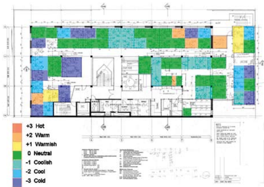
Figure 2 A study of a Government office floor highlighting the wide variety of comfort experiences.
