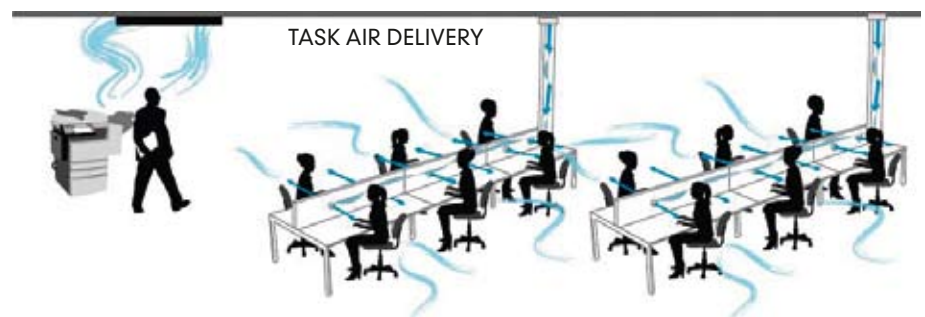
Figure 1 The concept is to bring a portion of conditioned air down through a duct to an adjustable diffuser built into the workstation.
