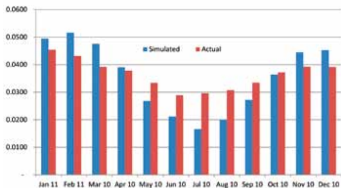
Figure 7: Main Fans kWh/sq.m.day
